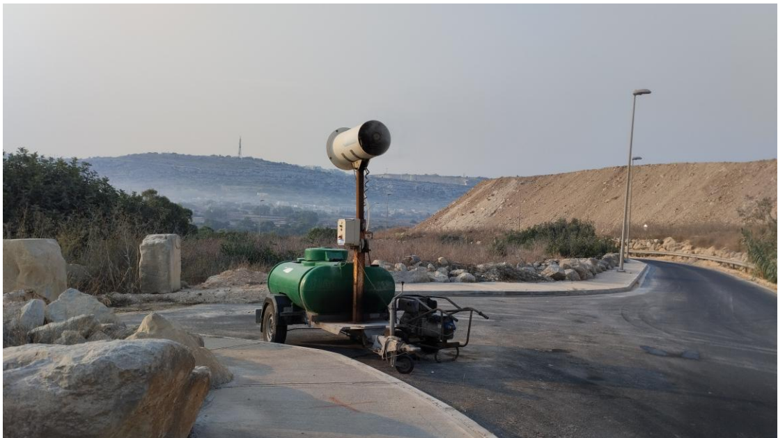
Figure 6: Mobile atomiser misting system within the internal access road of the ECOHIVE complex (25 th August 2023)
